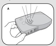
A Ensure Base Station and PIR Motion Sensor are in close proximity to each other. Press and release learn button on Base Station. Buzzer will sound.
